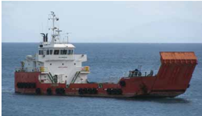
MV Seawind LOA 46m/Beam 10.9m/Max Draft 2.5m
